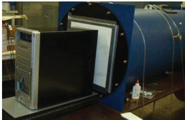
Figure 3. Chassis attached to the Airflow Test Chamber.
